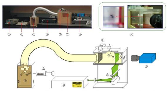
1. Delay & Pulse Generator @- Syringe Pump @-Fog Generator @- Nd:YAG Laser @- 3D Traverse @-Test Chamber @-Light Sheet Optics @- Digital Camera @- Fire Ant Alate
