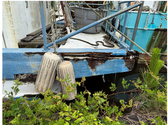
Figure 2. Close-up of “glass on wood” boat in severe disrepair. Note the wood is now exposed.
